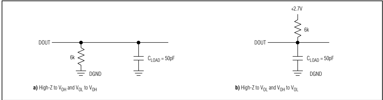
Figure 1. Load Circuits for DOUT Enable Time
