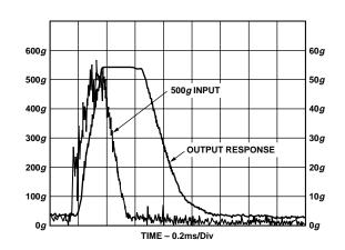
Figure 8. Typical 500 g Step Recovery at the Output
