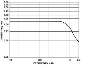
Figure 11. Noise Spectral Density
