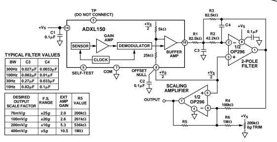
Figure 21. Two-Pole Post Filter Circuit
