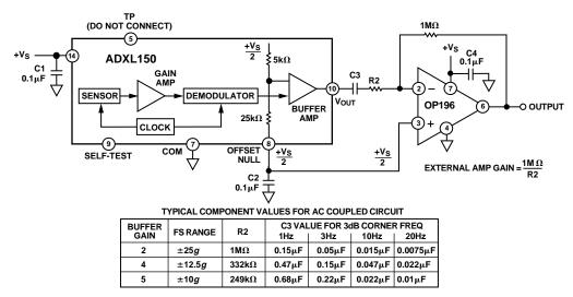
Figure 16. AC Coupled Connection Using an External Op Amp
